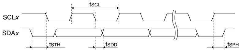
特記なき場合:  $V_{DD} = 1.8\sim 3.6V$ ,  $V_{SS} = 0V$ ,  $T_a = -25\sim 70^{\circ}C$
